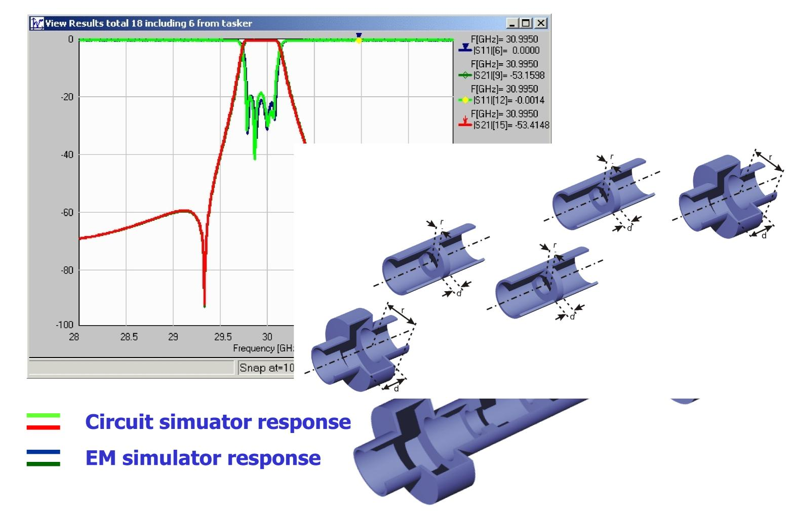
Rectangular waveguide filter with frequency-dependent couplings and its response computed by QW-3D and by circuit simulator based on models extracted from EM simulation.
