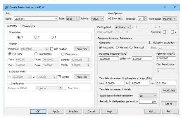
We set the name of the port to *LoadPort*. The default *Type* and *Orientation* of the port are properly set for this case. We should change *Activity* to MINUS (please note that when *Full Plane* option is checked, port will change its position to the opposite side of the project). We uncheck the *Reference* option – it is not necessary since we do not calculate S-Parameters.
