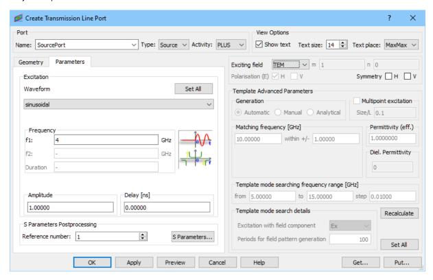
In the *Parameters* tab we set sinusoidal excitation at 4GHz. We excite the structure with a fundamental TEM mode. Pressing *OK* button accepts the settings.
