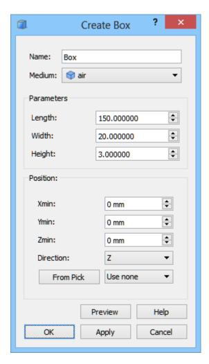
From the *Medium* combo box we choose air. Now we can proceed to setting the transmission line dimensions according to the picture above. With *Position* set to (0,0,0) the transmission line will be drawn so that its lower right corner is placed at this coordinates. After pressing *OK* button the transmission line object appears in the project.
