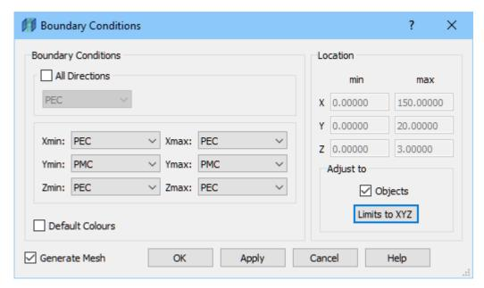
In the *Boundary conditions* frame we uncheck the *All* directions check box and we set *Perfect Magnetic Conductor (PMC)* for *Ymin* and *Ymax* positions and *Perfect Electric Conductor (PEC)* for the rest and press *Apply*. Please note that boundary conditions' indicators are visible when *Boundary Conditions* dialogue is opened or when visibility for *Computational Borders* is enabled. We will make
