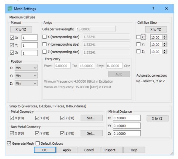
We set 1mm cell sizes in X, Y and Z direction. The meshing will be enforced in the entire project space.
