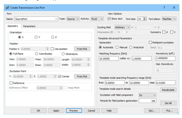
We set the name of the port to *SourcePort*. The default *Type, Activity* and *Orientation* of the port are properly set for this case. *Full Plane* option sets the port dimensions equal to the bounding dimensions of the entire project in the directions perpendicular to the port orientation what is suitable in this case. We uncheck the *Reference* option – it is not necessary since we do not calculate S-Parameters.
