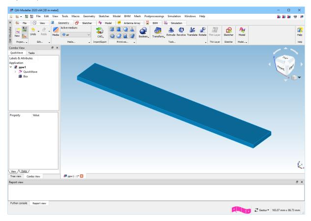
For better visualisation of the inside of the transmission line, we change its transparency by selecting *Box* object on the *Tree View*, and changing *Transparency* in the *View* tab in *Property Editor* to 50.
