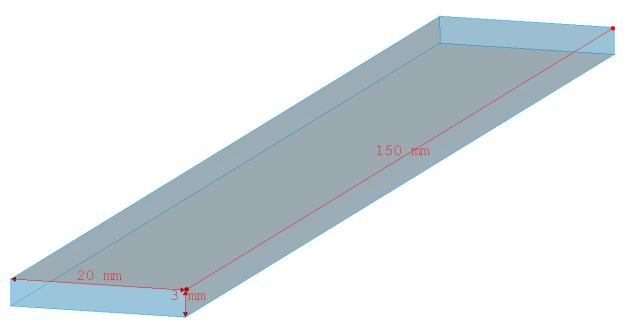
To draw the structure we go to *Geometry* tab. We start from drawing the transmission line inside filled with air. We need to draw only the inside of the structure (the surrounding medium is metal), thus we start from the air block, which stands for the transmission line inside. To draw the
