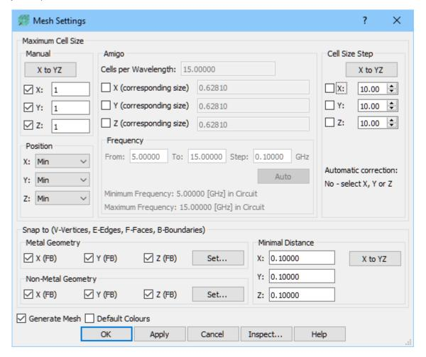
We set 1mm cell sizes in X, Y and Z direction. The meshing will be enforced in the entire project space.
