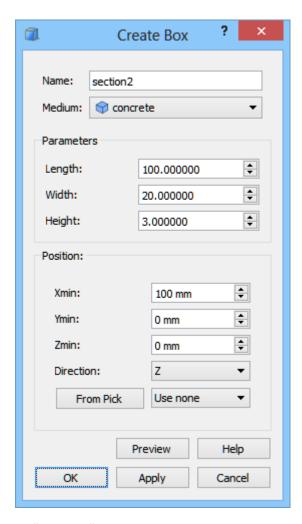
The name of this part is set to "section2" and its medium is chosen to be *concrete*. The dimensions of this part are the same as in the case of air filled section. The concrete filled part is placed behind the *section1* thus its position in X direction is set to 100 mm. After pressing *OK* button the concrete filled part of the transmission line appears in the project.
