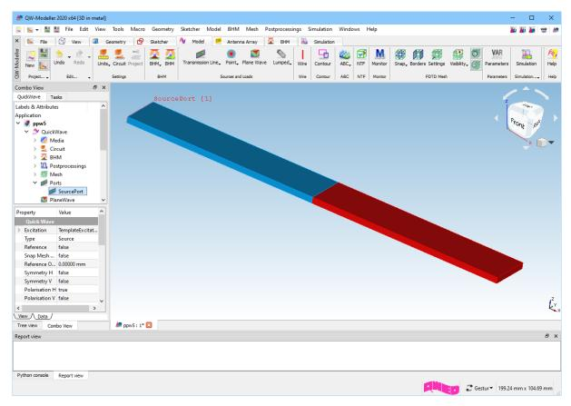
Now press Transmission Line Transmission Line commands button and choose Insert Transmission Line Insert Transmission Line Load... command.
