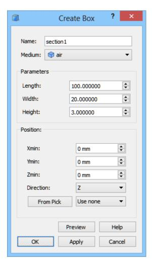
From the *Medium* combo box we choose air. Now we can proceed to setting the dimensions of the air filled part according to the picture above. With *Position* set to (0,0,0) the transmission line will be drawn so that its lower right corner is placed at this coordinates. After pressing *OK* button the air filled part appears in the project.
