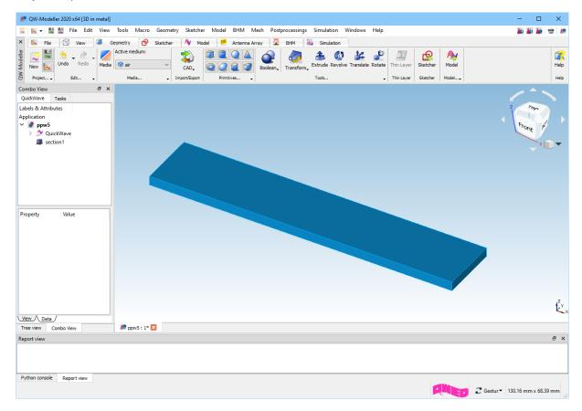
Before drawing the concrete filled part it is required to define concrete medium in the project. For
