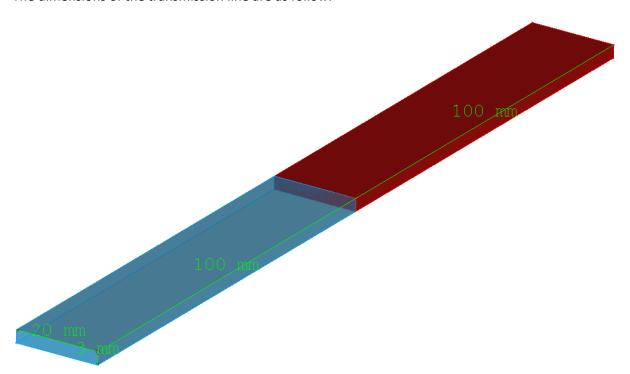
To draw the structure we go to *Geometry* tab. We start from drawing the transmission line inside. Firstly, the part filled with air is drawn. We need to draw only the inside of the structure (the surrounding medium is metal), thus we start from the air block, which stands for the first part of the
